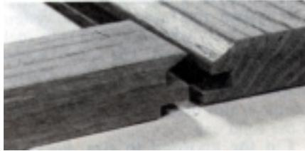
Once your rails and stiles have been cut and their edges created, slide a piece of 1/4" thick oak veneered plywood into the groove on the inside edges of your door frame pieces before gluing the stiles and rails together. **Do not glue the plywood panel to the rails & stiles.** No dowels will be necessary for assembly, since the cutters you use will create the proper corner joints for you.
